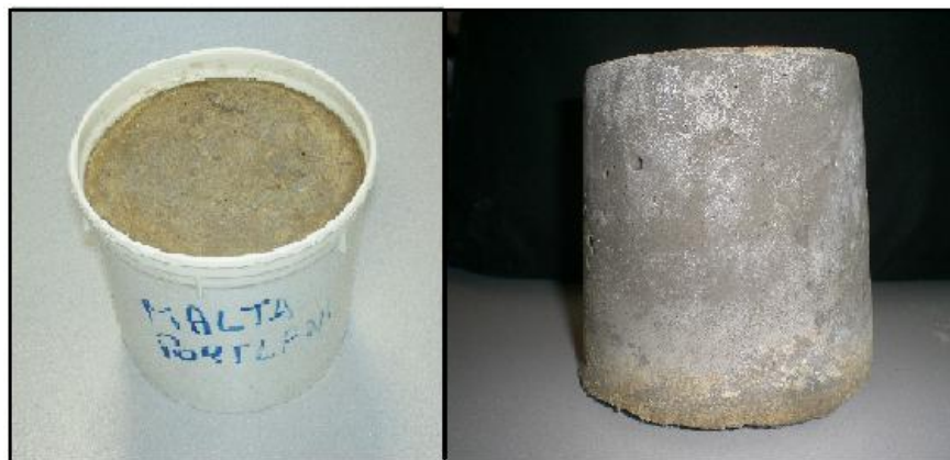
Figure 58 Sample cured in constant humidity conditions by Portland after 5 years of its preparation (MAPEI UTT, Personal Information).
