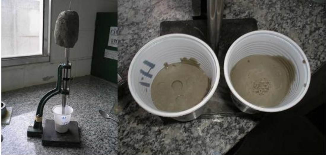
Figure 53 Modified Vicat apparatus /0,1 MPa compressive strength is achieved. (Pellegrini et al, 2009))
