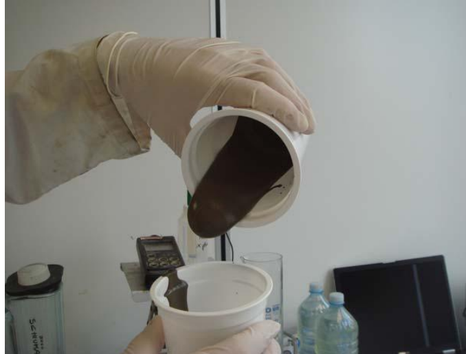
Figure 51 Sample after during the gel time test (Pellegrini et al, 2009)
