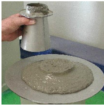
Figure 43 Inert Mortar Slump Test. (Linger et al, 2008)
