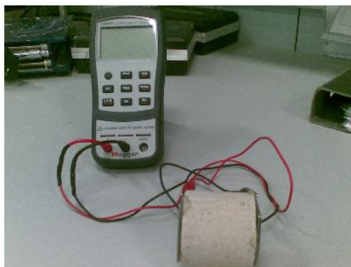
Figure 50 Resistivity Test execution (Cylinder 10) (Peila et al, 2008)
