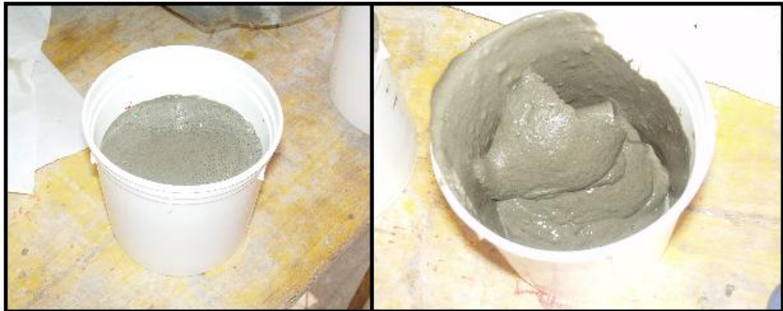
Figure 46 Sample before and after the gel time test
