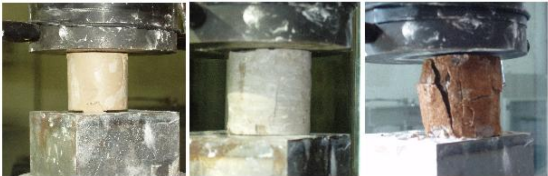
Figure 48 Compression Test. From left to right: Cylinder 8/ Cylinder 9/ Cylinder 12
