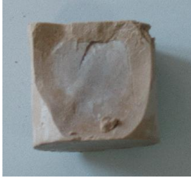
Figure 49 Water Absorption Test Sample (Cylinder 9). (Peila et al, 2008)
