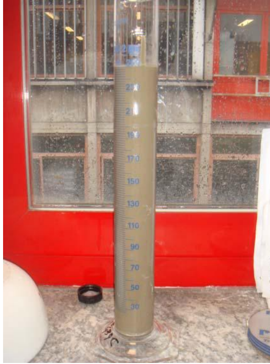
Figure 37 Used instrumentation for the bleeding test (Pellegrini et al, 2009)
