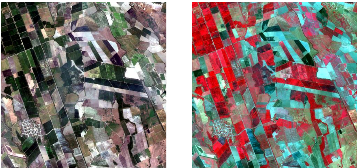
Figure 1 – Multispectral image of Turén, Portuguesa state, Venezuela, acquired by the Miranda satellite. Shown in true color at left and near-infrared color at right.
