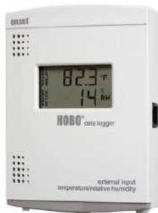
HOBO data logger. Tem/Rh/light/ext
