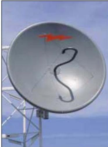
Standard Parabolic Antenna
