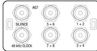
The AG7 provides eight channels (four AES/EBU pairs) of audio signal generation. It also provides two channels (1 AES/EBU pair) of silence as well as a 48 kHz clock output.
