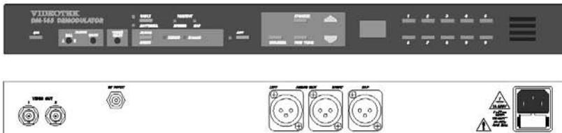
Like the DM-141A, the next model in the Videotek demodulator series, the **DM-145**, is perfect for broadcast and cable applications and adds the capability of providing both stereo audio and SAP (Second Audio Program) outputs. Second language programming, emergency alert, or radio simulcasting are a few of the applications that require full time SAP audio.
