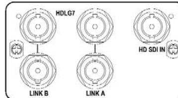
The HDLG7 is a test signal generator that provides two identical dual-link high-definition serial digital interface (HD SDI) outputs. The module supports video formats that require the use of a dual-link interface, such as 4:4:4 RGB at rates up to 1080i/60 Hz or 1080p/30 Hz or 4:2:2: YCbCr at rates up to 1080p/60 Hz. The HDLG7 supports several standard test signals and also has the unique ability to up-convert an arbitrary single-link HD SDI input signal to a dual-link format for the outputs.
