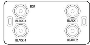
The BG7 is an analog black generator with four independently selectable outputs. The BG7 Black Generator supports NTSC and PAL black burst as well as HDTV tri-level sync. With Option CB, two of the outputs can also generate various analog NTSC and PAL color bar test signals.
