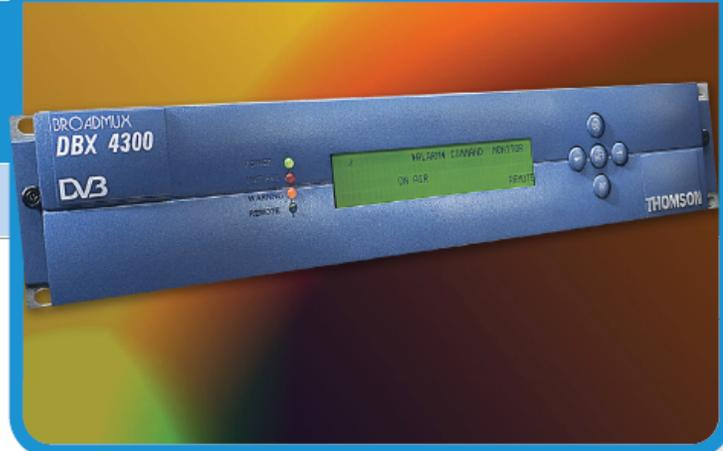
With the DBX 4300, Nextream provides operators with a leading re-multiplexing solution for composing a set of services for a digital television system. The DBX 4300 can handle up to 26 transport streams, ensuring full DVB of output streams. Broadmux also provides operators with a cost-effective solution for MPEG-2 local program insertions by using its integrated near seamless splicing.
