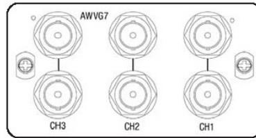
The AWWG7 is an Analog Wideband Video Generator that supports a variety of HD analog component formats (Y'P'bP'r or GBR). The module provides two identical component outputs with a bandwidth of 30 MHz. Up to two AWWG7 Analog Wideband Video Generators can be placed in a single TG700 mainframe.
