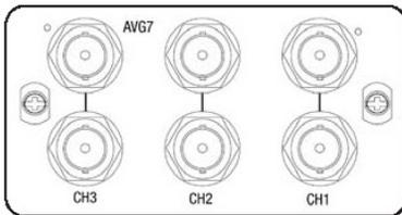
The AVG7 is an Analog Video Generator for 525/625 interlace formats supporting component (Y'P'bP'r; G,B,R, Y/C), 525 Beta, and composite (PAL, NTSC, NTSC NoSetup). It provides two identical component outputs, two identical Y/C and Composite or six identical composite outputs.
